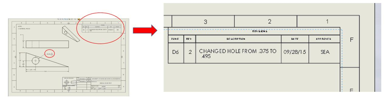
If the change to the part is severe enough that you could not install it on all assemblies back to the original usage, then change the part number, begin at the initial revision, and revise the assembly(s) it is used in. We often refer to this as violating "form, fit, or function".
