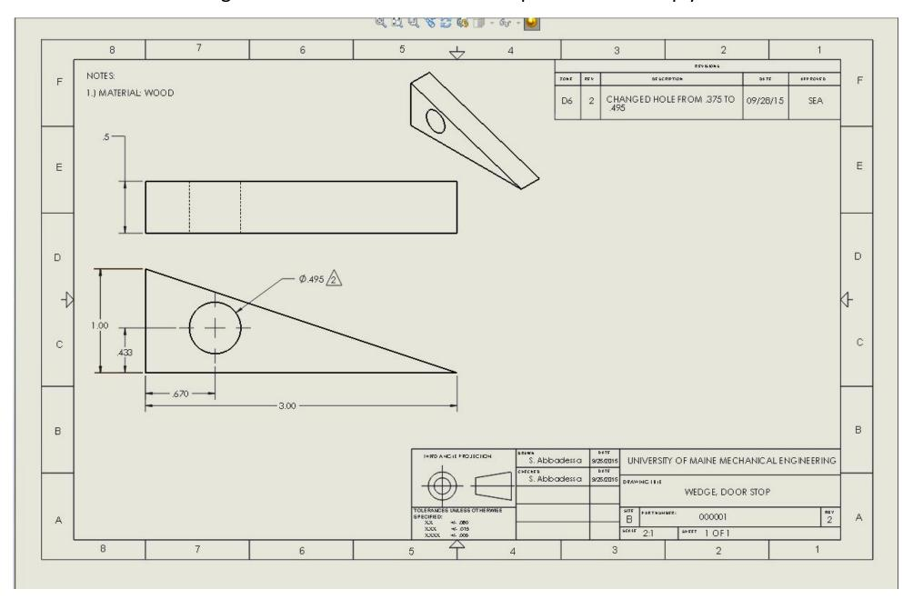
Not all of the six sides of the box need to be shown if the geometry can be fully described with fewer views.
