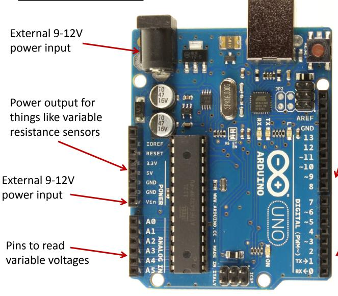
Digital input/output pins. Use these to signal to turn things on or off, read if a switch is open or closed, etc.
